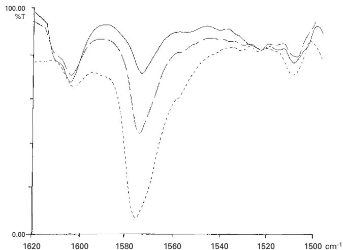
Fig. 5 IR spectra in the \text{Ag}(\nu_{12}) region band: (....) DMAN, (-----), 2:1 complex and (—) 1:2 complex.
